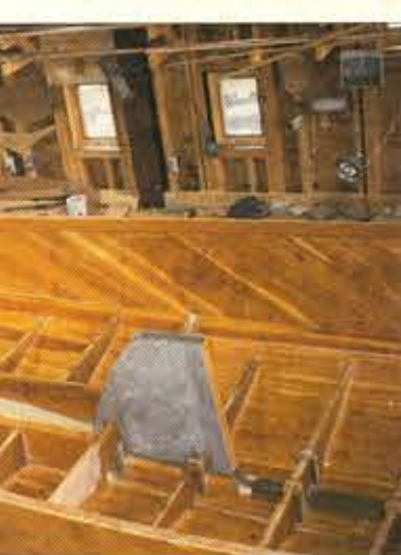
Top left: Having planked up the boat upside, Dr Chile Crisler and friends turn it over for fitting out.
