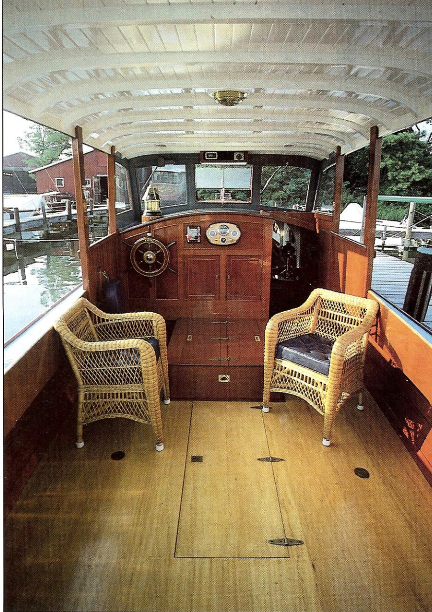
View of the cockpit, looking forward, with new white mahogany sole, fresh paint and varnish, and wicker furniture in place.
